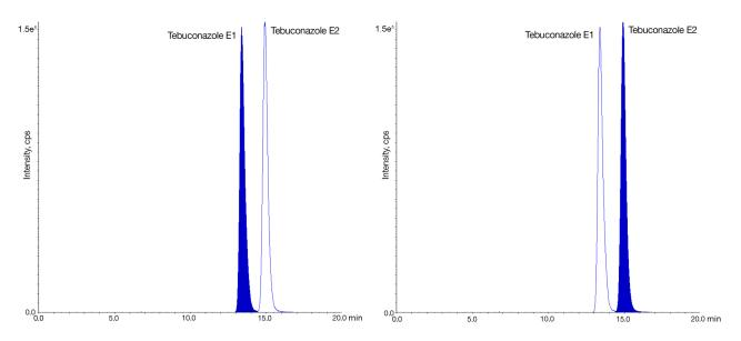
Figure 7: 250 µg/L Standard Solution; Separation of Tebuconazole enantiomers on **CHIRAL ART Cellulose-SC** (KSC99S03-1503WT, 3 µm particle size, 150 mm × 3 mm), 0.43 mL/min, 25°C, 1 µL injection volume, water with 0.1% formic acid/acetonitrile (60/40), ESI+ m/z 308-70.
