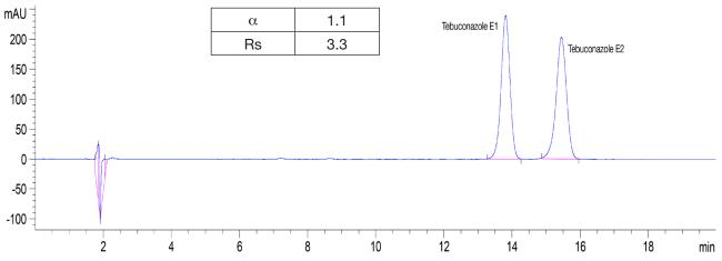
Figure 6: Separation of enantiomers Tebuconazole on **CHIRAL ART Cellulose-SC** (KSC99S03-1503WT, 3  $\mu$ m particle size, 150 mm × 3 mm), 0.43 mL/min, 25°C, 2  $\mu$ L (1 mg/mL) injection volume, water with 0.1% formic acid/ acetonitrile (60/40), 220 nm.
