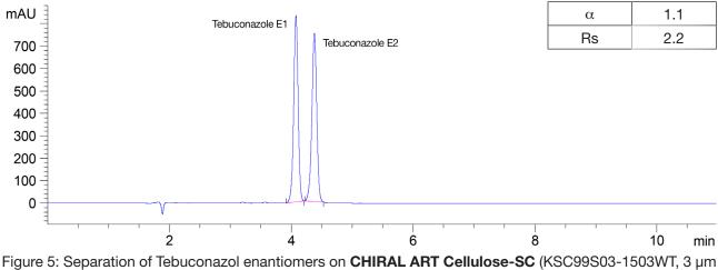
Figure 5: Separation of Tebuconazol enantiomers on **CHIRAL ART Cellulose-SC** (KSC99S03-1503WT, 3 μm particle size, 150 mm × 3 mm), 0.43 mL/min, 25°C, 2 μL (1 mg/mL) injection volume, water with 0.1% formic acid / acetonitrile (40/60), 220 nm.
