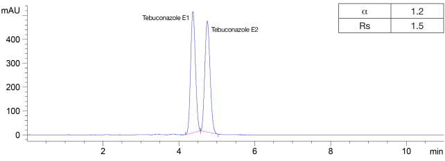
Figure 3: Separation of Tebuconazol enantiomers on CHIRAL ART Cellulose-SC (KSC99S05-1546WT, 5  $\mu$ m particle size, 150 mm × 4.6 mm), 1 mL/min, 25°C, 5  $\mu$ L (1 mg/mL) injection volume, water/acetonitrile (40/60), 220 nm.
