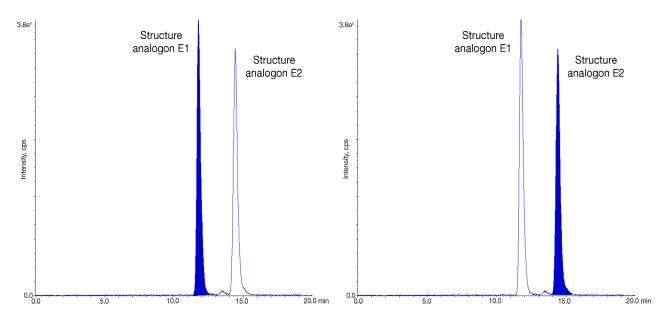
Figure 8: Separation of structure analogon enantiomers on **CHIRAL ART Cellulose-SC** (KSC99S03-1503WT, 3  $\mu$ m particle size, 150 mm × 3 mm), 0.43 mL/min, 25°C, 1  $\mu$ L injection volume, water with 0.1% formic acid/ acetonitrile (60/40); ESI+ m/z 312-70.
