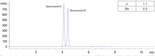
Figure 4: Separation of Tebuconazol enantiomers on **CHIRAL ART Cellulose-SC** (KSC99S03-1503WT, 3  $\mu$ m particle size, 150 mm × 3 mm), 0.43 mL/min, 25°C, 2  $\mu$ L (1 mg/mL) injection volume, water/ acetonitrile (40/60), 220 nm.
